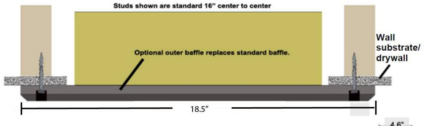
Pixel Pro can be ordered with an oversized outer baffle to allow for in-wall installation.
