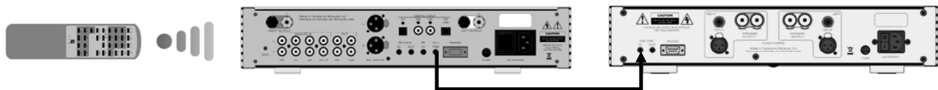
Figure 6: Remote Operation with 12V Trigger
