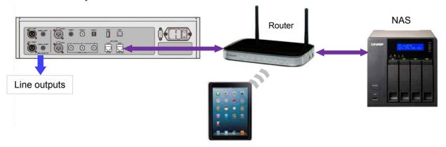
Figure 3 – Using a **Bartók DAC** with a NAS
