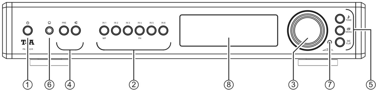
All the important functions of the **PA 2000 R** can be controlled using the buttons and rotary knob on the front panel. Direct-acting buttons are provided for fundamental functions such as source selection. Functions which are needed less frequently are controlled using menus which are called up by pressing the **MENU** / **FLAT** button.
