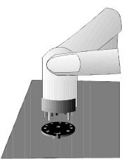
**4.** After you've examined all the tubes to make sure that they are firmly placed in their sockets, you can put the protective cage back onto the amplifier unit. Tighten the screws to make sure that the cage is securely fastened to the unit.
