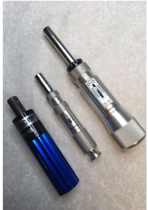
Recommended top quality torque drivers left: fixed torque middle and right: adjustable torque
