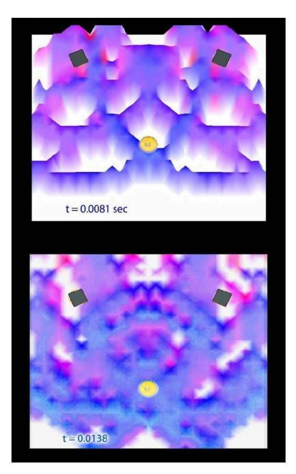
After less than 1/100<sup>th</sup> of a second, the room has developed a complex wave pattern with energy varying with room position. The listener is now awash in a series of wave-fronts which will soon reflect off the wall behind.
