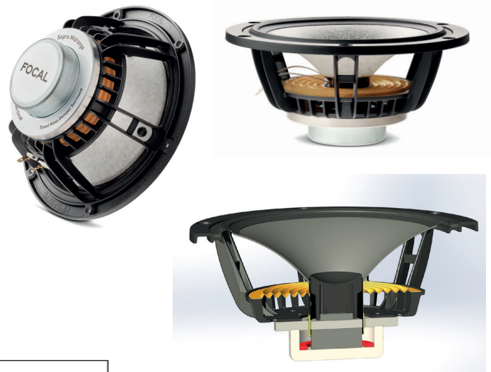
Fig L: Our simulation tool has led us to this optimized «NIC» magnetic circuit for the midrange driver. It reconciles efficiency with linearity of the voice coil inductance as a function of both the position of the coil and the current flowing through it, across the frequency range.
