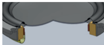
Fig K: Magnetic circuit without a pole piece. Focal patent US 2013/0064413
