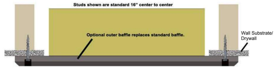
After positioning the speakers, use a drywall saw to cut an opening slightly larger than the 12.15" x 35.5" cabinet body.
