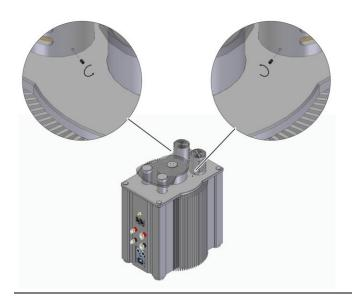
Remove the grounding screws using the Allen key supplied.
