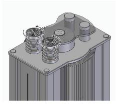
Loosen the tube covers by turning them counterclockwise and then remove them upwards.
