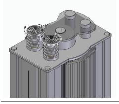
Tighten the tube cover clockwise.
