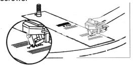
VTA Adjustment: The VTA for the installed Ortofon cartridge has been properly set at the factory. To adjust the VTA for other cartridges, lay a record on the platter (2). Slacken the horizontal adjustment screws (two Allen screws located near the plinth on the back of the tonearm pillar) with the Allen Key provided.
