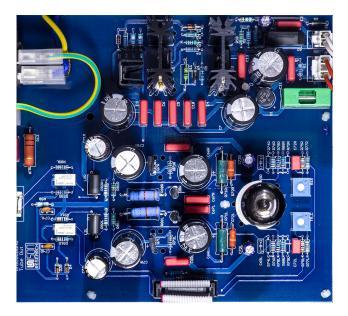
The audio stage is designed around a single 12AU7//ECC82 double triode operating in pure class A, defining the sonic performance of the unit, followed by a solid state discrete buffer still operating in class A for a low impedance output and ideal audio behaviour. The totem pole circuit is also used in the One and 150 in the Only 90 of the same line of CDdue.
