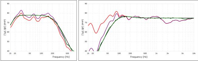
The red curves represent the in-room response before correction, as an average from five measurement positions, whereas the green ones show response with equalization applied. In this case a subwoofer and bass management are also in use. In the subwoofer graph, which is on the left, the difference between the level of the red and purple curves shows the amount of room gain.
