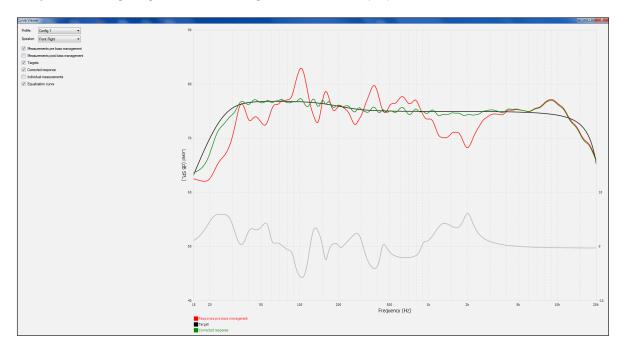
In contrast, this is the same measurement with the original targets that were automatically detected and set by ARC. Notice how the left side of the target curve complies to the speaker's natural rolloff:
